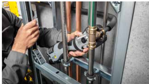
The Pressgun Picco 6 Plus excels when space is limited and enables single-handed pressing in any situation.
